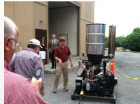
Syngas Generator using wood chips
