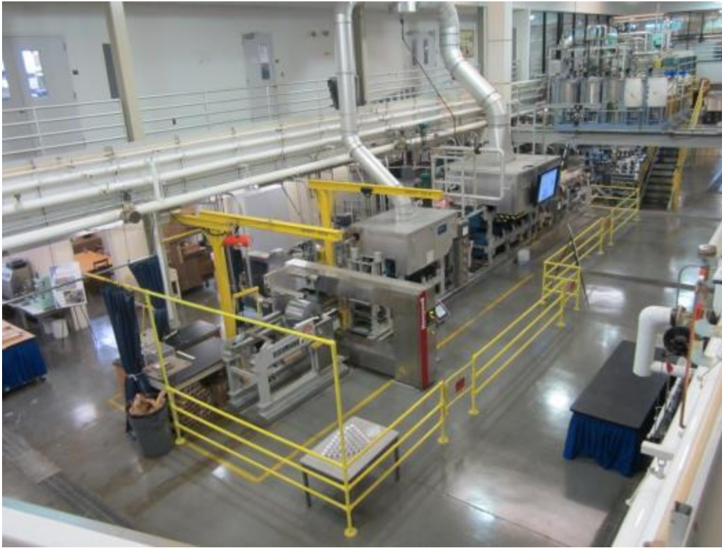
Pilot paper machine with advanced control systems
