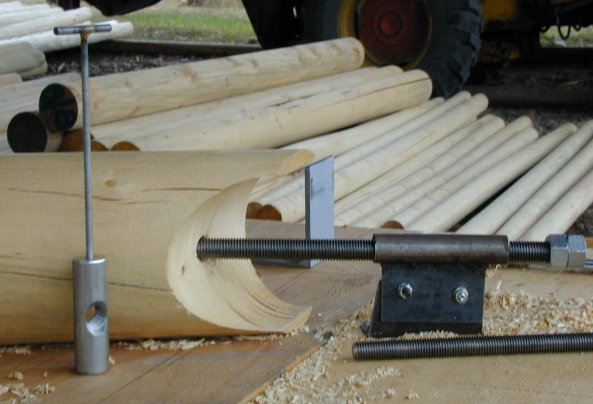
Strong connectors can pull timbers together
