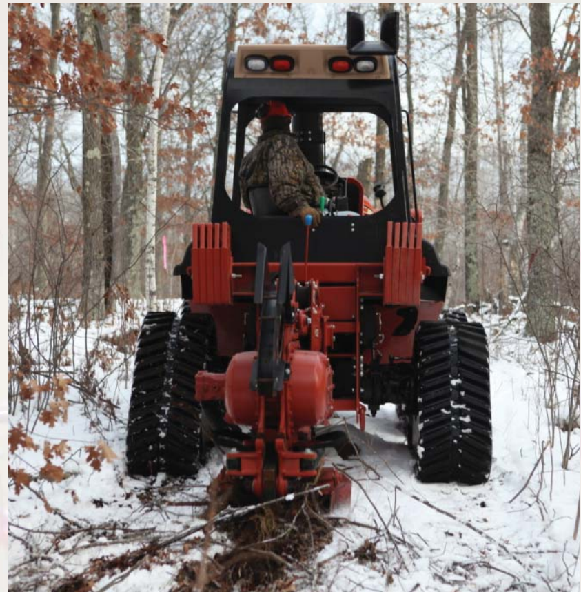
Department of Natural Resources fire officers install root graft barriers with a vibratory plow in Menominee County.
